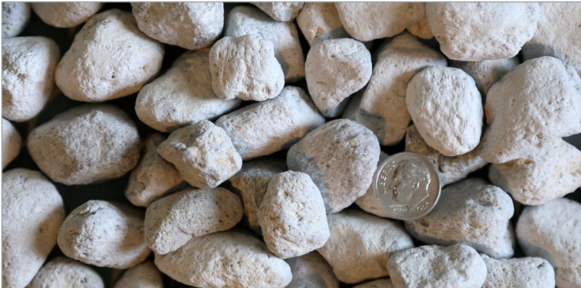
HP Grade one by three-quarters inch stones dried and free of fines.
